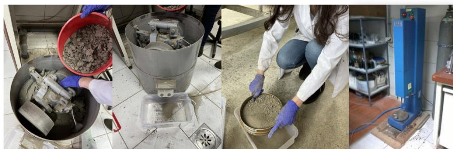
Figure 1. Steps in the stabilization/solidification process
