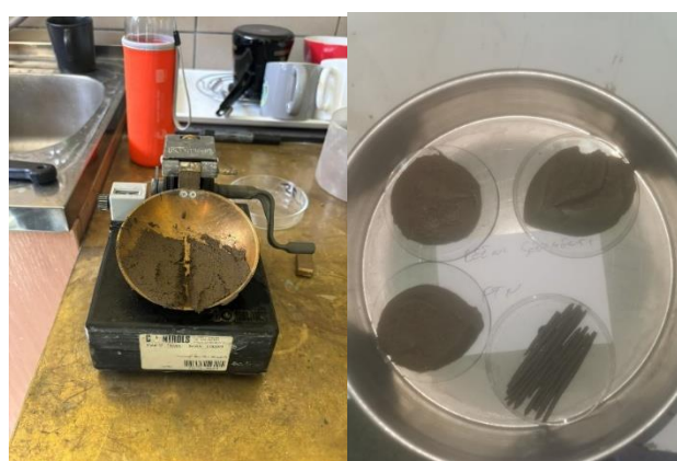
Figure 3. Yield strength (left image) and plasticity limit (right image)
